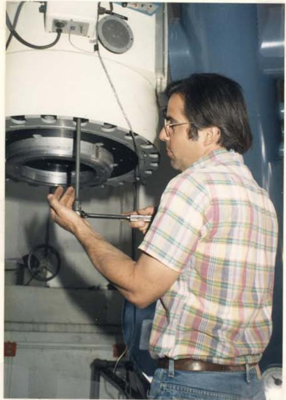
*Remove all but three allen head bolts that hold cell on. Leave three that can be removed with fork lift in position.*
