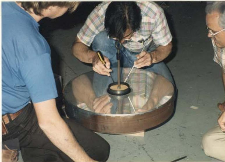
Support center assembly from bottom and remove ring ball retainer from the top of the balls.
