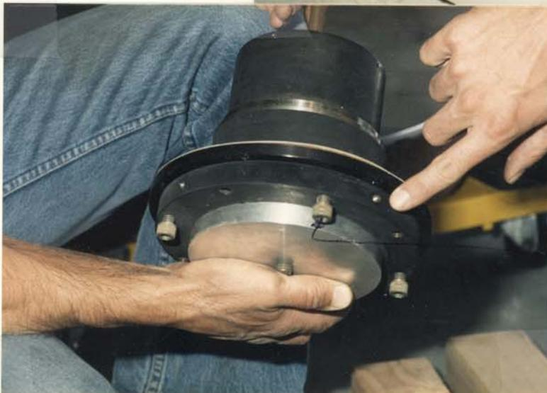
To remove mirror from cell first loose 2 of 4 centering screws (reach from inside center hole)
